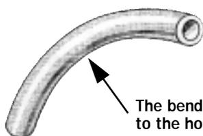
The bending radius is measured to the hose inside.
